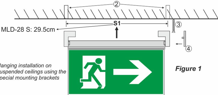
*Hanging installation on suspended ceilings using the special mounting brackets*
