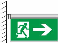
Flag mounted installation on a wall using the special mounting bracket contained in the package.
