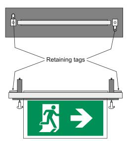
4. Fasten the two retaining screws clockwise and the retaining tags will expand until the base is securely installed.
