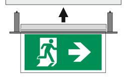
3. Push upwards the base. Make sure that the retaining tags are not expanded.
